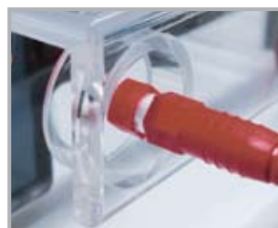
Safety lid offers protection against electric shock
