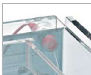
End Gates for leak proof sealing of the gel tray
