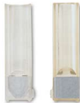
External and internal V-shaped profile of the cuvette
