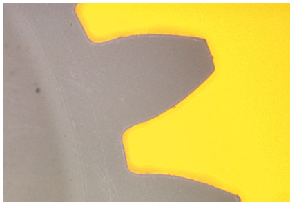
Plastic Gear Teeth with Smaller Module
