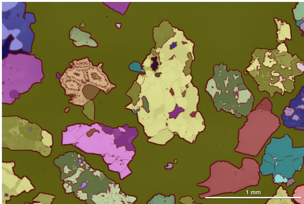
Feature-based image segmentation of a geological sample.
