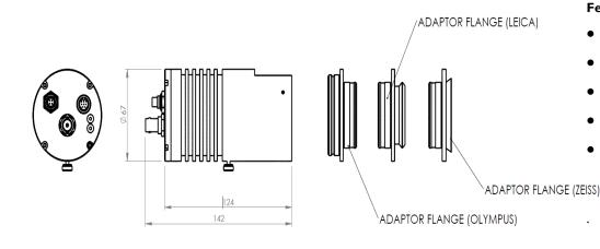
Brightfield LED illuminator provides all the advantages of LED illumination in a flexible package that can be fitted to most modern microscope systems, both inverted and upright. This compact device fits easily to the microscope, simply replacing the standard lamp house, but the LED will provide 10,000+ hours of operating lifetime.
