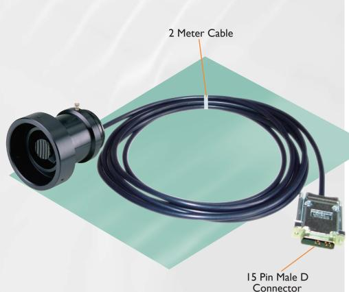
The motorized focus control from Prior Scientific provides step sizes as small as 0.002µm give excellent resolution for precise focus and repeatable positioning in the Z-axis. For large movements when speed is required, the ProScan focus motor can be driven at speeds of up to 20 revs/s. An optional probe style encoder feedback system provides the highest accuracy and repeatability available.
