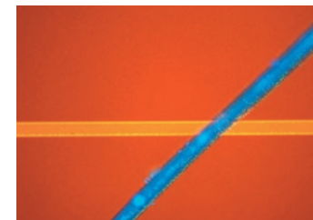
Epi-fluorescence observation of organic substance on wafer
