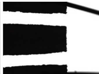
Lead frame Episcopic illumination at optical magnification 4x
