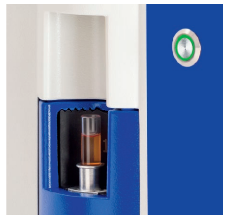
Figure 1: the Lumat has a motor-driven revolving magazine mechanism for convenient sample switching.
